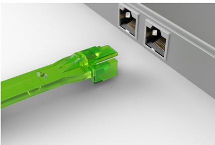
**1.** A lock is attached to the key and inserted into an RJ-45 port.
